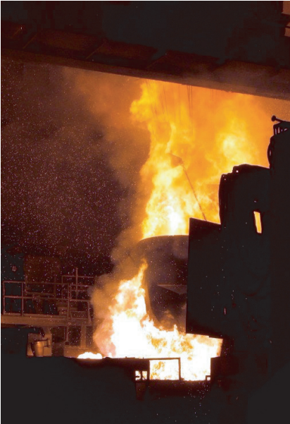
44 tons of scrap are melted every 57 minutes into molten steel in the melting pot. The table roller bearings the melting pot is seated on are lubricated with Molyslip High Temperature Bearing Grease .
